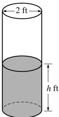
4. A cylindrical barrel with a diameter of 2 feet contains collected rainwater, as shown in the figure above. The water drains out through a valve (not shown) at the bottom of the barrel. The rate of change of the height  $h$  of the water in the barrel with respect to time  $t$  is modeled by  $\frac{dh}{dt} = -\frac{1}{10}\sqrt{h}$ , where  $h$  is measured in feet and  $t$  is measured in seconds. (The volume  $V$  of a cylinder with radius  $r$  and height  $h$  is  $V = \pi r^2 h$ .)
